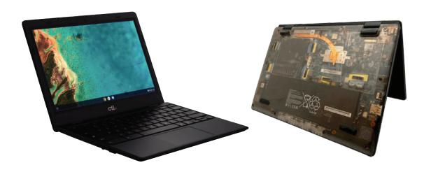
The PX11E "Secure" special edition is a Chromebook with a semi-transparent bottom, secured with anti\_tamper security screws that allows visibility into the electronics inside the device
